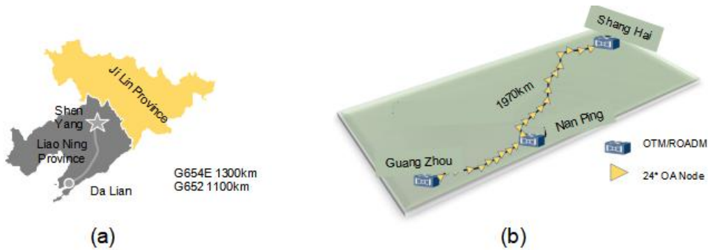
Figure 4.1. 400G Transport Path in the Existing Network: (a) Dalian – Shenyang Path of China Mobile; (b) Guangzhou – Shanghai Path of China Telecom
