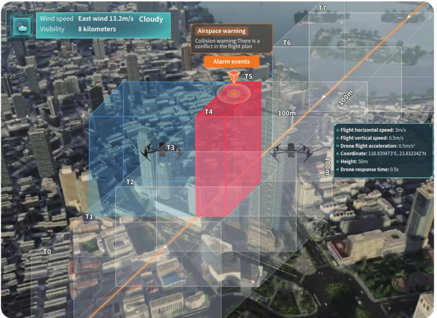
Figure 21: Collision buffer zone effect of UAV
