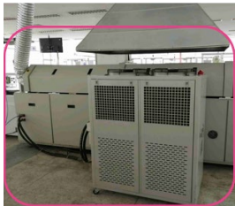
Water-cooling system transformation of the REHM reflow furnace.
