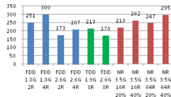
Fig. 1A. Comparison of UL coverage at the edge rate of 2 Mbps.
